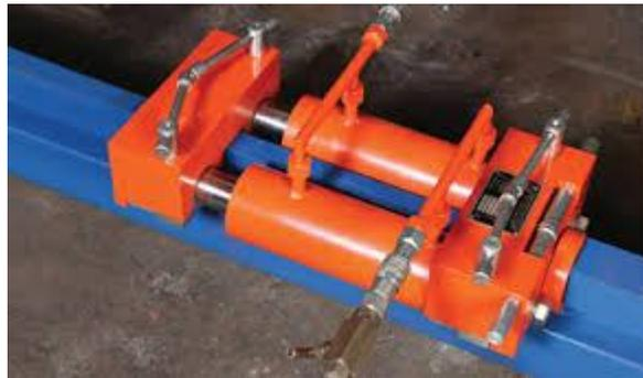
**Hydraulic Tank & Roof lifting Jacks**
